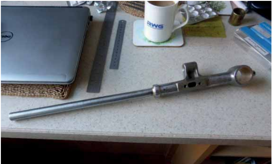
Repaired handbrake lever ready for painting
