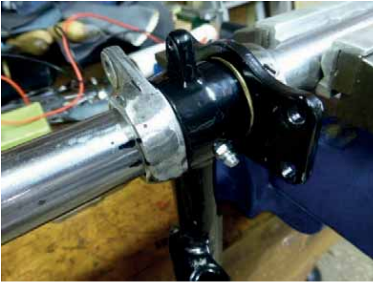
Re-assembly in progress - ready for welding
